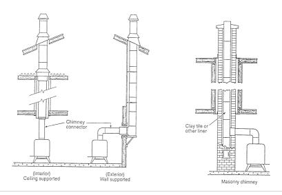
Be sure that all connectors between the chimney parts and the heater are sealed properly so the chimney is airtight from the heater to the chimney outlet.
