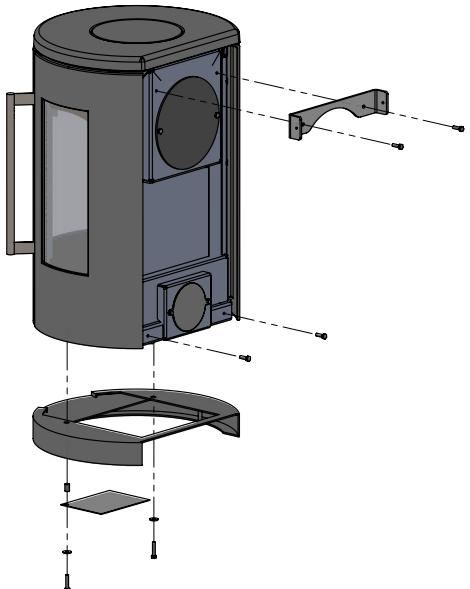
Lift the stove body into place so that the 2 x M8 screws under the base of the stove line up with the oval holes on the wall bracket.
