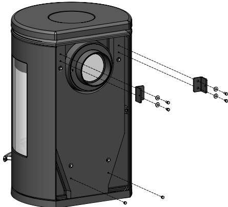
The basic oven is lifted into place, so that it sits on the bottom of the wall mounting. The oven must be fixed using the 2 pcs. M5x12 screws supplied at the top and the 2 pcs. M8x16 screws and washers supplied at the bottom (see sketch). We recommended that 2 persons should carry out this work.
