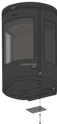
Mount the CE label underneath the stove as shown. Use the included screw with washer.
