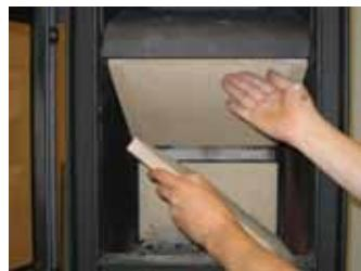
4. Once the side brick panels have been removed, lower the bottom baffle and lift it out.
