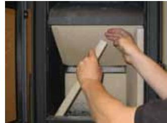
3. Tilt one of the side brick panels and remove it.
