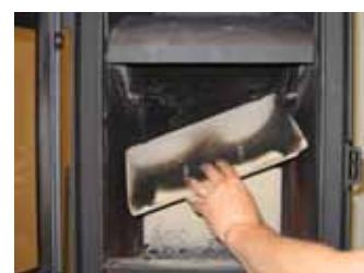
6. Make sure that the baffles and brick panels are correctly assembled before lighting the stove after cleaning.
