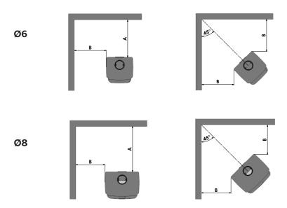
In situations where the stove is to be fitted into a brick or non-combustible recess, we recommend that the stove is installed with at least 10 cm clearance to the wall, this will allow room air to circulate around the stove; also the maintenance of the outside stove is easier. When applied to masonry, a layer of wallpaper is normally classified as a non-combustible surface.
