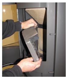
4. Lift the bottom baffle plate again and tip the other brick panel out.
