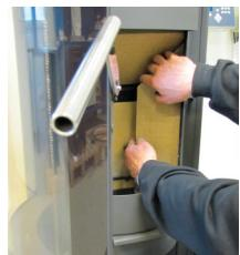
5. Lift the bottom baffle plate free of the tertiary combustion air box and remove it.
