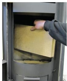
6. If necessary, the rear brick can now be removed.
