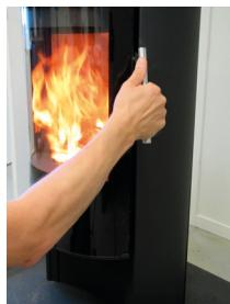
5. Re-stoking should normally be carried out while embers still remain. Distribute the embers in the bottom, ensuring that most of them are at the front of the stove.
