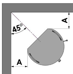
We recommend that the stove be installed at least 10-15 cm from masonry in order to allow heat to circulate and to facilitate the cleaning of the inside and outside of the stove. A layer of wallpaper on a brick wall is normally regarded as non-flammable material.
