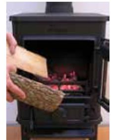
6. Lay three pieces of wood (see dimensions above) onto the embers. Leave half an inch (1 cm) or more between each piece. Place the ends of your logs towards the opening, but not too close to the front.
