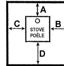
FLOOR PROTECTOR MUST BE NON-COMBUSTIBLE MATERIAL. IT MUST EXTEND BENEATH HEATER, AND TO THE FRONT/SIDES/REAR AS INDICATED.
