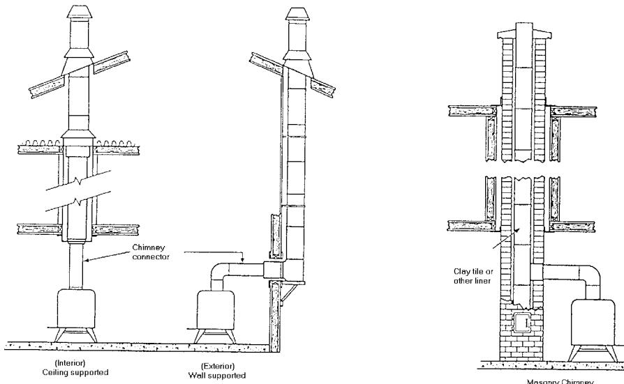
Be sure that all connectors between the chimney parts and the heater are sealed properly so the chimney is airtight from the heater to the chimney outlet.
