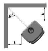
In situations where the stove is to be fitted into a brick or non-combustible recess, we recommend that the stove is installed with at least 10 cm clearance to the wall, this will allow room air to circulate around the stove; also the maintenance of the outside stove is easier. When applied to masonry, a layer of wallpaper is normally classified as a non-combustible surface.
