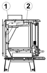
Make sure that the baffle plate (2), the fire bricks and the riddling are positioned correctly.
