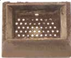
Burn pot with holes clogged with ash. Must be cleaned
