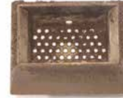
Burn pot with holes clogged with ash. Must be cleaned
