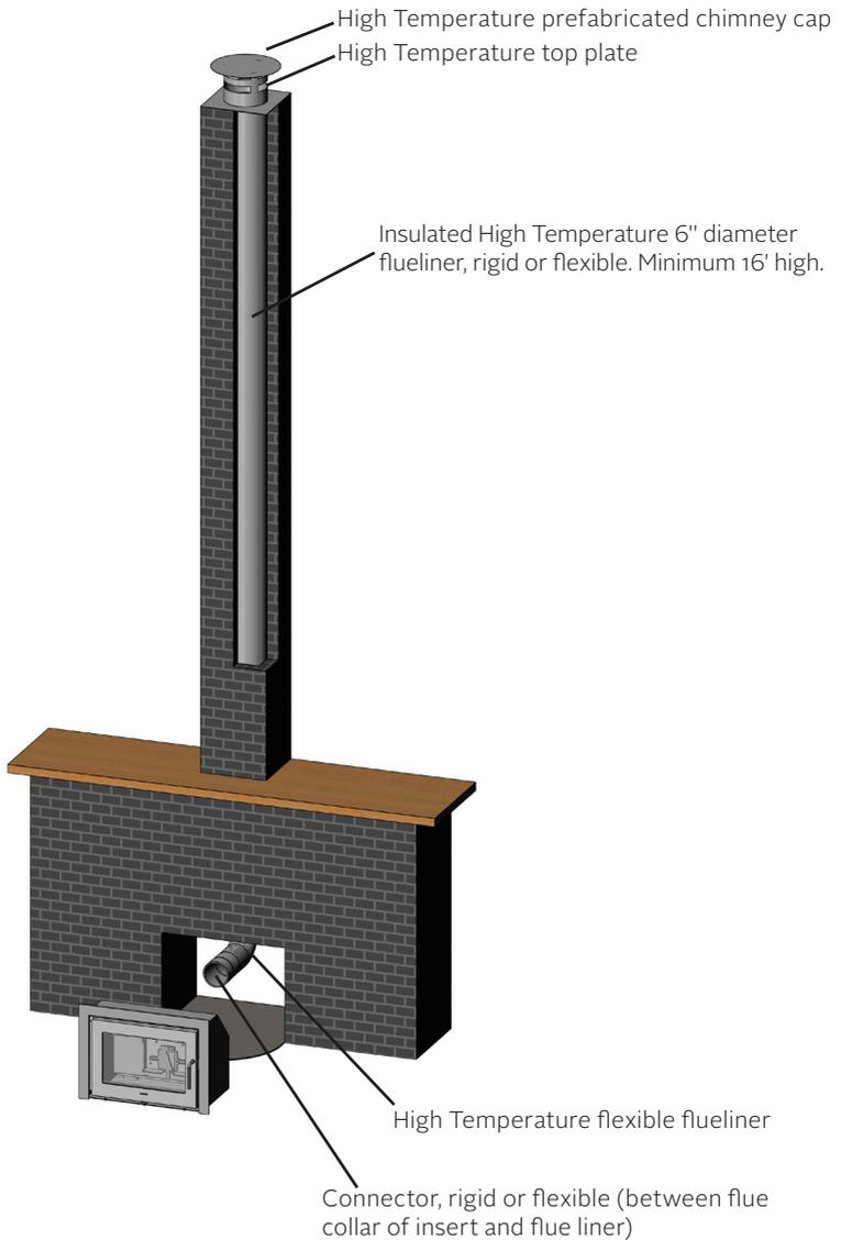
Sample installation into existing chimney.
