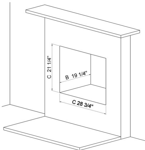
The figure above shows the required fireplace dimension required for the Morsø 5660 Standard insert.
