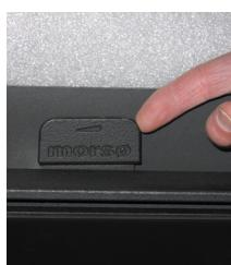
The stove door should normally be opened gently the first 2-3 cm, then you should wait until the pressure has equalised before opening the door all the way. This technique will prevent smoke from getting out, particularly when there is a poor draught.
