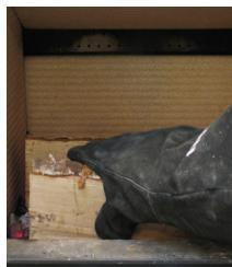
7. When the secondary air supply is opened to maximum and the door is closed, the new quantity of wood will ignite in a few minutes.
