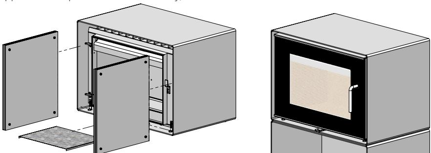
For wall-mounted installation, the modules can be levelled off by way of the supplied adjusting screws and and levelling feet with the Allen key (see sketch). When the installation of the combustion chamber and the flue-duct arrangement is completed, continue by mounting the side modules, if relevant. Please note that, for safety reasons, no module is allowed above the combustion-chamber module.
