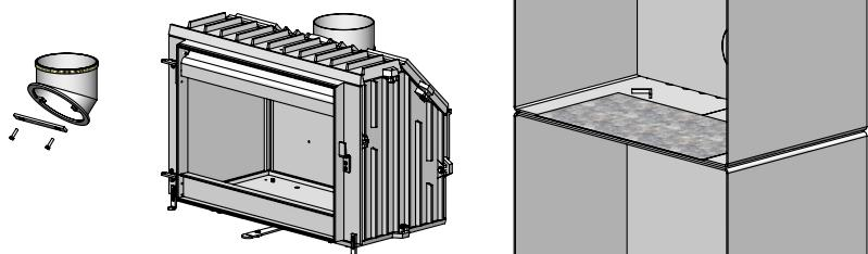
Now, place the lower radiation screen in its approximate position below the combustion chamber, and the 2x3 sets of radiation plates (supplied in assembled states) are placed in their approximate positions – one set each side (see sketch). Avoid pushing them all the way up against the rear plate of the module. Next, the vermiculite plates are refitted, the upper vertical plate as the last. Finally, the door is remounted.
