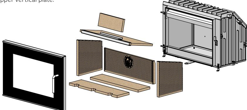
**NOTE! WHEN FITTING OVENS WITH TOP-MOUNTED OUTPUT, THE FLUE DUCT CANNOT BE FITTED BEFORE THE OVEN HAS BEEN INSERTED INTO THE MODULE.**
