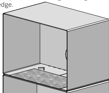
Dismantle the door from the oven and remove the vermiculite plates, beginning with the upper vertical plate.
