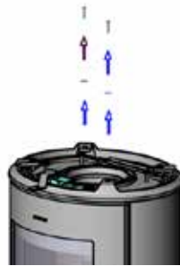
Flue to the rear
