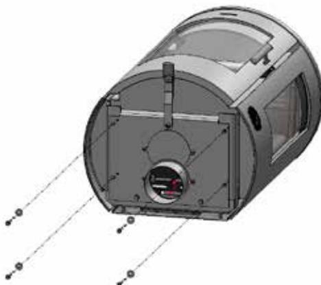
Finally, re-install the drawer using the four screws previously removed.
