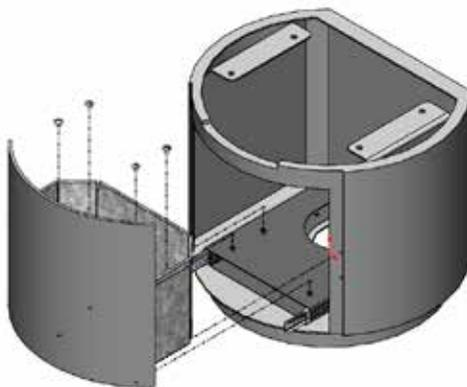
The heat screen supplied with the drawer is installed at the same time as screwing on the plinth. (see sketch).
