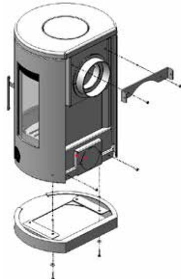
The basic oven is lifted into place, so that its sits on the bottom of the wall mounting. Assemble the stove using the 2 no. M6x12 screws supplied at the top and the other two M6x25 screws and washers which were previously removed at the bottom. (see sketch). We recommended that 2 persons should carry out this work.
