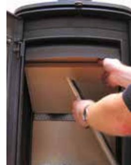
4. Once the side brick panels have been removed, lower the bottom baffle and lift it out.
