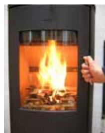
5. If the condition in step 4 is met, place max. 3 pieces of wood with a total weight of 1.5-2.5 kg and a length of 25-30 cm over the embers in a single layer, with a distance of approximately 1 cm.
