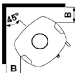
We recommend that the stove be installed at least 10 - 15 cm from masonry, in order to allow heat to circulate and to facilitate the cleaning of the inside and outside of the stove. A layer of wallpaper on a brick wall is normally viewed as non-flammable material.
