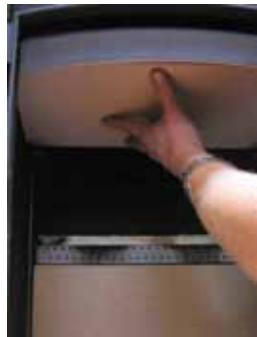
6. Make sure that the baffles and bricks are correctly reassembled before lighting the stove after cleaning.
