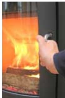
7. Reduce the amount of combustion air to the desired position, and the optimal combustion will continue. Make sure that there is always enough air (oxygen) to maintain clear, lasting flames when, and after, reducing the amount of combustion air.
