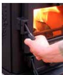
8. Once the new fuel has taken, adjust the secondary air amount to the desired setting; optimal combustion will continue until glowing charcoals are produced. Under normal chimney draft conditions, expect to refuel your stove every 60 - 70 minutes.
