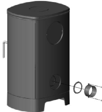
The base connecting air kit consists of an air box with spigot, sealing gasket and two M6 x 30mm screws and washers. Seal the self adhesive gasket around the circular hole on the inner face of air box. Slide the air box up from the base of the stove and secure with the two fixing screws.
