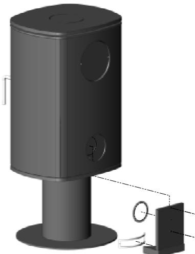
When fixing the direct air supply to the pedestal stove the air kit consists of an air box, sealing gasket and two M6 x 30mm screws and washers. Seal the self adhesive gasket around the rectangular hole at the top of the pedestal and the circular hole on the inner face of air box. Slide the air box up from the base of the stove and secure with the two fixing screws.
