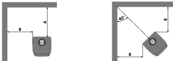
In situations where the stove is to be fitted into a brick or non-combustible recess, we recommend that the stove is installed with at least 10 cm clearance to the wall, this will allow room air to circulate around the stove; also the maintenance of the outside stove is easier. When applied to masonry, a layer of wallpaper is normally classified as a non-combustible surface.
