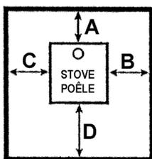
Floor protector must be non-combustible material, with an R-value of 1.0. It must extend beneath heater and to the front/sides/rear as indicated.
