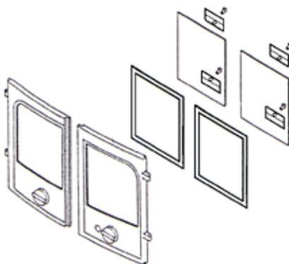
1. Lift the door off its hinges and place face-down on a sheet of cardboard or other non-abrasive fabric.
